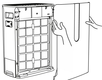
2. Replace the primary filter. Hold down the buckle, pull out, remove the filter at the bottom of the main groove, close the filter.
