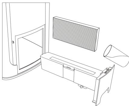
3. Replace the filter. Pull out the filter by the tip, then you can replace the carbon cloth mesh filter.
