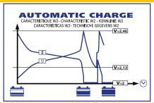
Charge to 100% lead or liquid batteries (Curve W2) from 40Ah to 350Ah.
