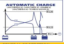
• Charge to 100% lead or liquid batteries (Curve W2) from 35Ah to 150Ah.
