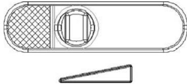
To operate the fireplace at the minimum output, set the primary air supply control to fully closed position. If you have a fluepipe damper installed, close the damper as well.
