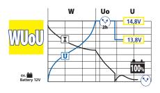
• Charge to 100% lead acid, gel, calcium and AGM start/stop batteries (Curve WuoU) from 25 to 180Ah.
