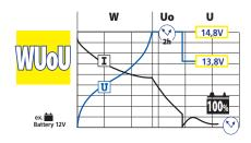
• Charge to 100% lead acid, gel, calcium and AGM start/stop batteries (Curve WuoU) from 20 to 150Ah.
