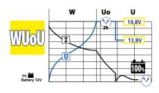
• Charge to 100% lead acid, gel, calcium and AGM start/stop batteries (Curve WuoU) from 15 to 100Ah.
